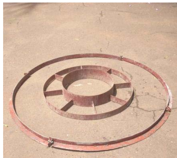
Picture 4: Fully Assembled (Outer & Inner) Mould for Dome Slab
