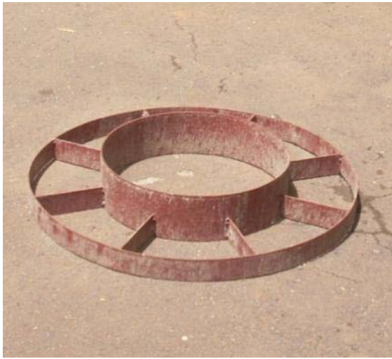
Picture 1: Inner piece of the dome slab mould
